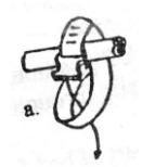
2. Snap two parts of the Quick Release Buckle together. Verify buckle is securely snapped.
